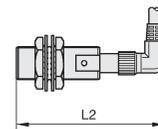
When using an angled connector, dimension L2 is the overall length plus 20 mm.
