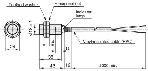
Vinyl-insulated cable (oil-resistant: 0.5 mm<sup>2</sup>, 45/0.12 dia., 2-core) dia. 6. Cap color: orange.
