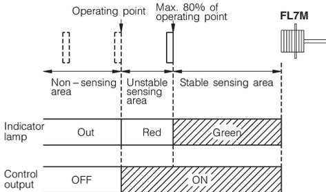
**Note:** When the target object is made of a different material such as aluminum, copper and stainless steel to the standard target object (iron), the setup point where the indicator lamp changes color is shorter than 80% maximum.
