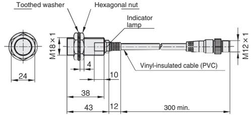
Vinyl-insulated cable (oil-resistant: 0.5 mm<sup>2</sup>, 45/0.12 dia., 2-core) dia. 6. Cap color: orange.
