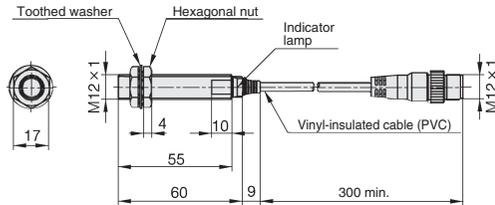
Vinyl-insulated cable (oil-resistant: 0.3 mm<sup>2</sup>, 60/0.08 dia., 2-core) dia. 4. Cap color: orange.
