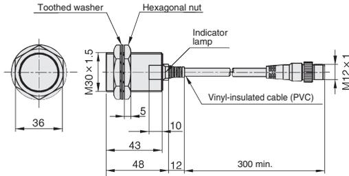
Vinyl-insulated cable (oil-resistant: 0.5 mm<sup>2</sup>, 45/0.12 dia., 2-core) dia. 6. Cap color: orange.
