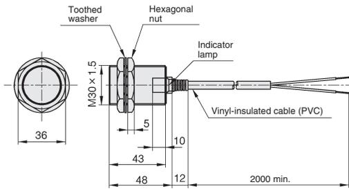
Vinyl-insulated cable (oil-resistant: 0.5 mm<sup>2</sup>, 45/0.12 dia., 2-core) dia. 6. Cap color: orange.
