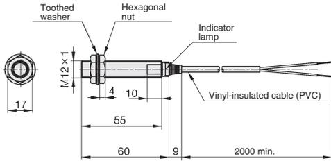
Vinyl-insulated cable (oil-resistant: 0.3 mm<sup>2</sup>, 60/0.08 dia., 2-core) dia. 4. Cap color: orange.
