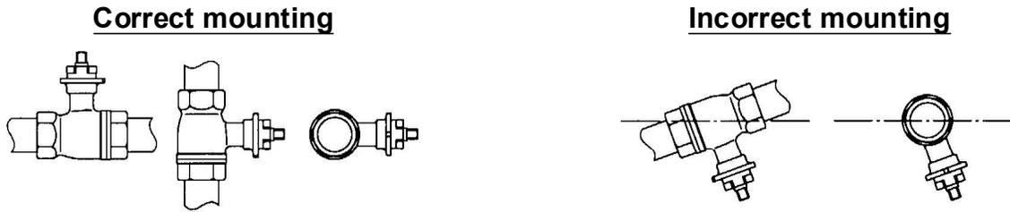
Figure 4. Mounting positions of the valve
