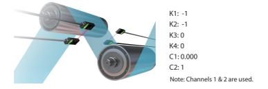
Calculating the average of channels 2, 3, and 4 and the difference between the average and channel 1.
