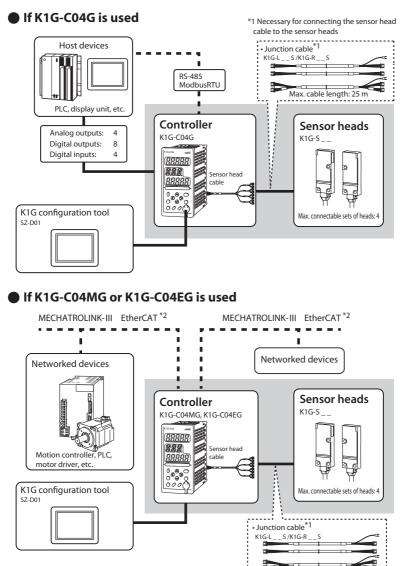
\*1 Necessary for connecting the sensor head cable to the sensor heads
