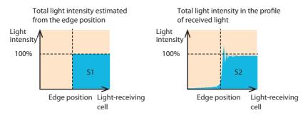
If there is a shadow in the profile of received light due to a smudge on the light-receiving surface, S2 will decrease, and thus the light intensity change rate will be lower.
