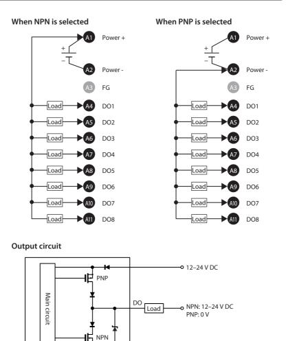
Output current (source or sink): 1 to 10 mA (per output)ON-state voltage drop:2 V max.OFF-state leakage current:0.3 mA max.Common type:8 (shared with power terminals)
