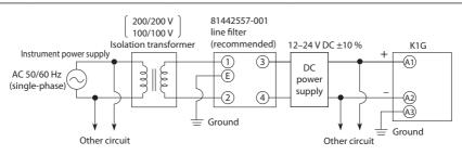
Use the frame ground terminals of this device (A3 and the network frame ground terminals\*) for one ground connection only. Do not run wiring across to other terminals. If it is difficult to wire the shielded cable, etc., use a separate ground terminal (earth bar).
