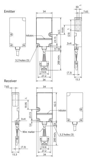
\*<sup>1</sup> Total light emission area:  $23(H) \times 6(W)$ \*<sup>2</sup> Center of the measurement width
