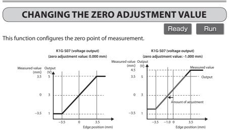
After the zero adjustment, change the analog output (AO) range so that the analog output correctly corresponds to the measured value. CP. 4-25
