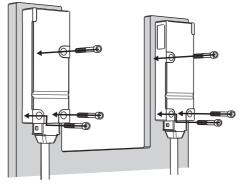
Tightening torque: 0.5 N·m max.
