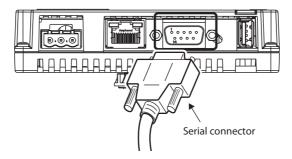
**2** Connect the loader cable jack to the loader port on the controller
